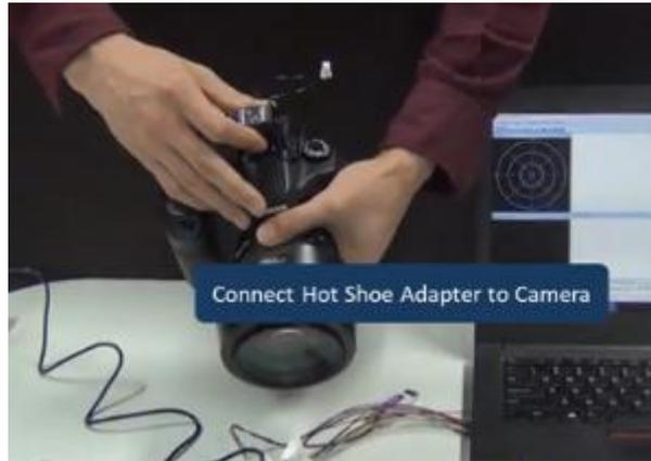
Figure 2.3 Connect hot shoe adapter to the camera
