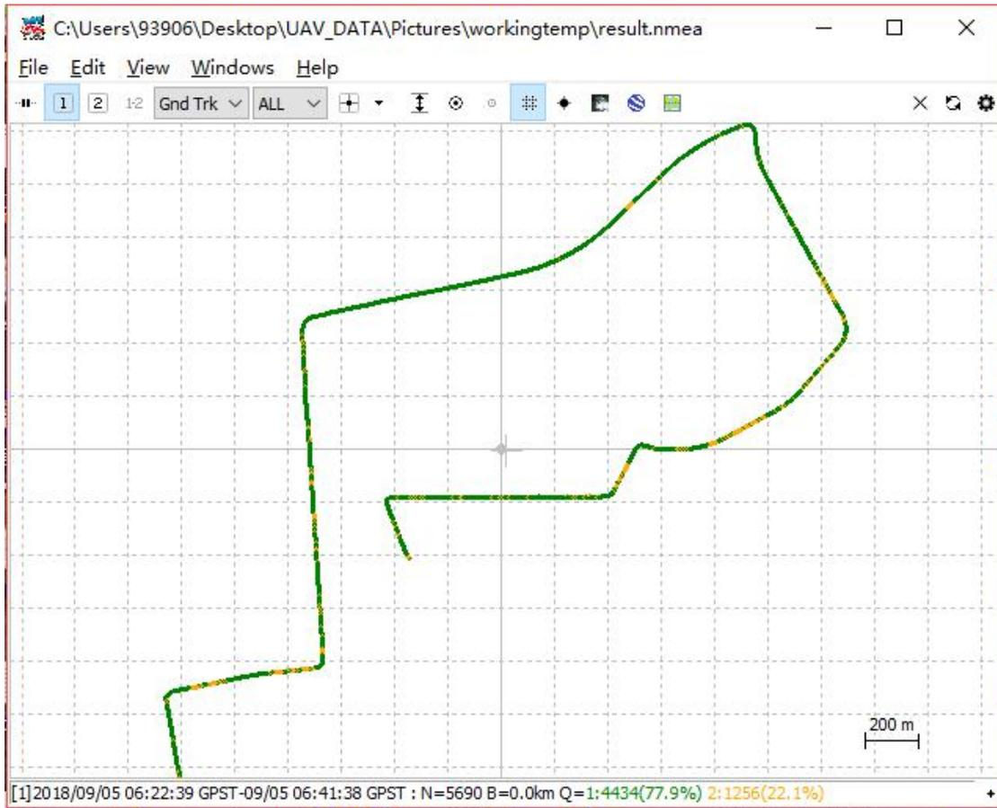
Figure 6.11 Positioning results of the GNSS post-processing
