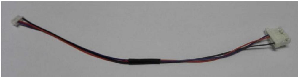
Figure 5.22 Cable between Pixhawk and BX306
