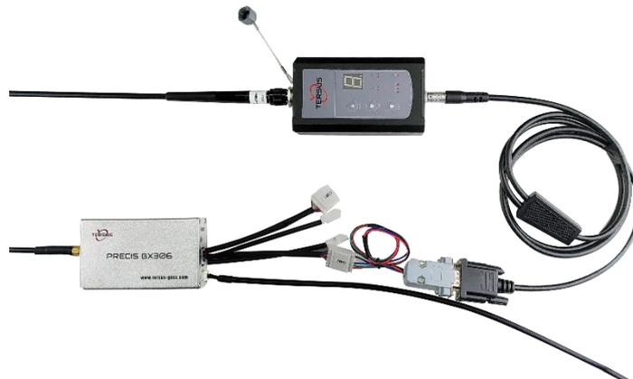
Figure 5.21 Outline of BX306 Connected to RS460 Radio
