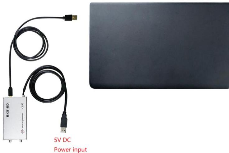
Figure 2.10 BX316D Enclosure connected to a Laptop
