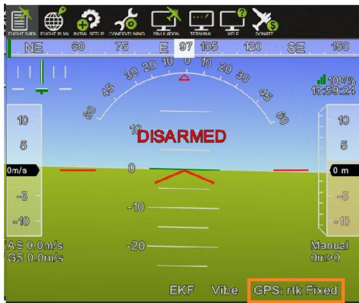
Figure 5.26 GPS status changes to rtk Fixed
