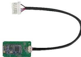
Figure 5.8 BT120 and the cable
