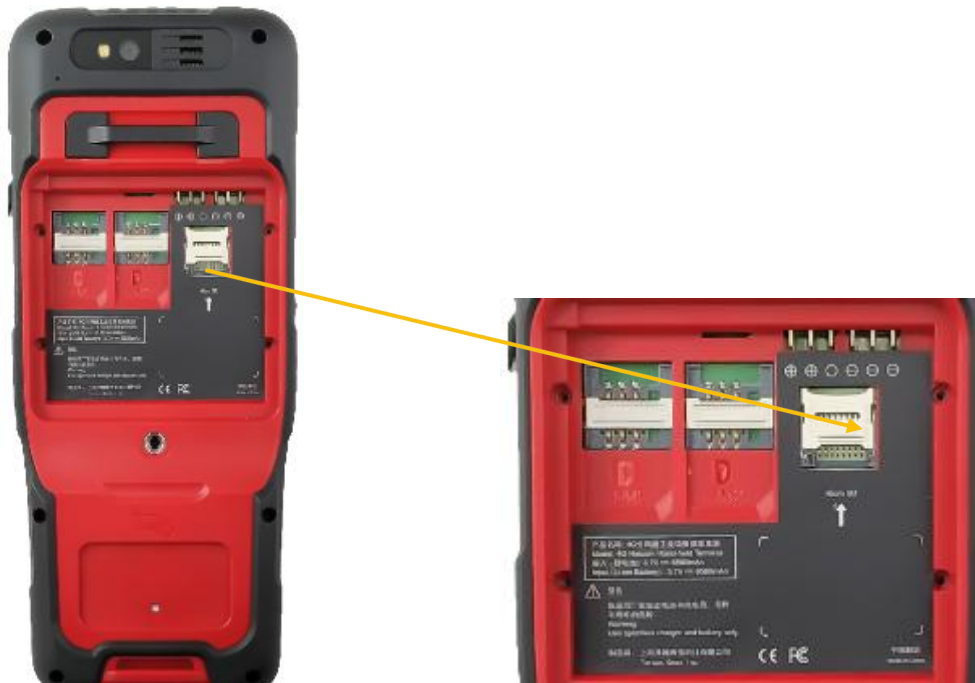
Figure 6.10 Insert Micro SD card
