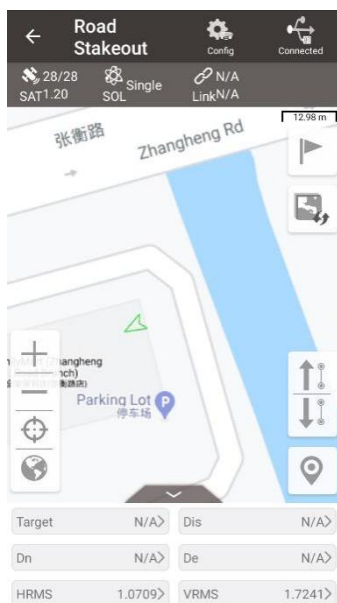
Figure 4.66 Road stakeout interface
