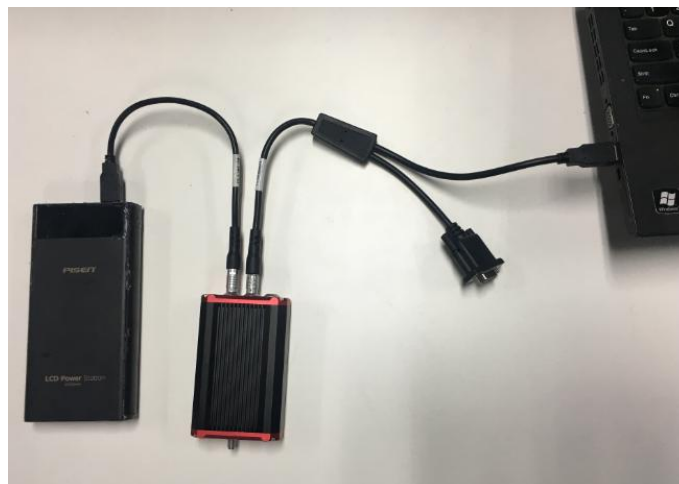
Figure 4.35 Connections of David, computer and power bank
