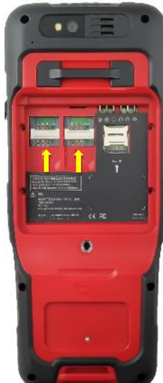
Figure 6.9 Put the SIM card in the holder
