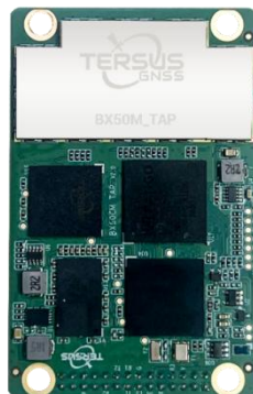
Figure 1.2 The BX50M-TAP Board
