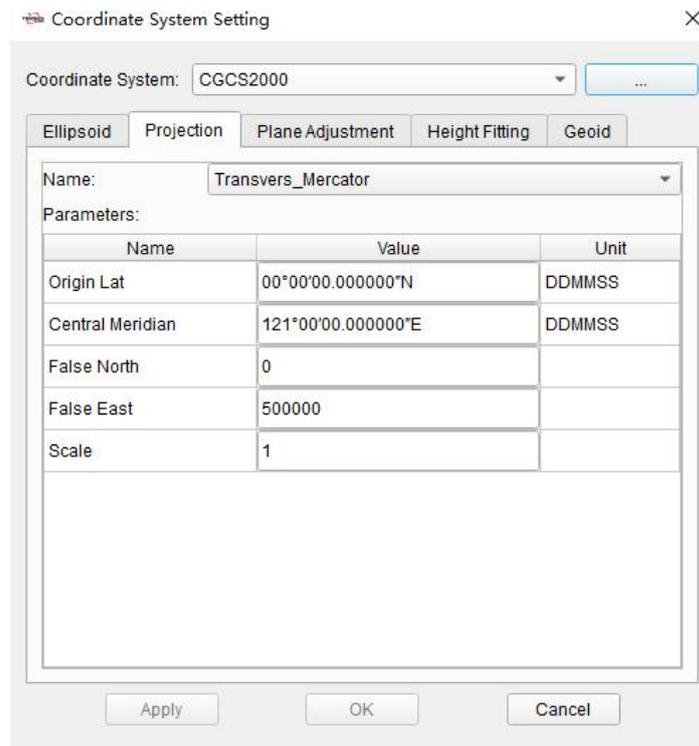
Figure 2.3 Quick Start - Edit Coordinate System
