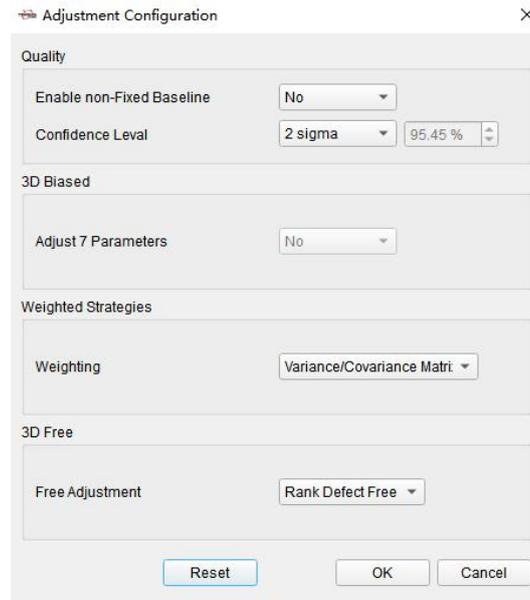
Figure 6.16 Adjustment Configuration
