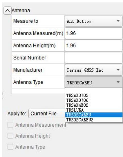
Figure 6.6 Antenna Parameters Modifying
