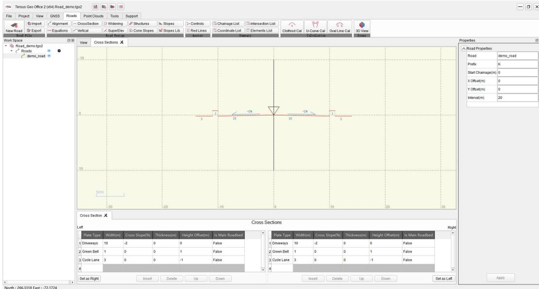
Figure 2.12 Quick Start - Road Cross Sections Parameters Editing
